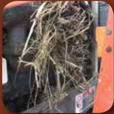
Tractor owners face very real dangers during this peak season. Fires can start when nesting material is placed on an already hot surface, but more typically fires start when the tractor resumes operation.
